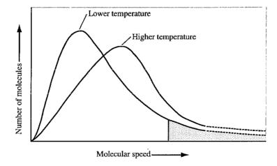
In both cases the average speed of the molecules is proportional to temperature. The distribution of molecules becomes broader as the temperature increases. This means that there are a greater number of molecules traveling within a greater range of higher speeds as the temperature increases.
