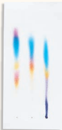
FIGURE A Paper chromatography reveals the different colored dyes that black ink contains.
