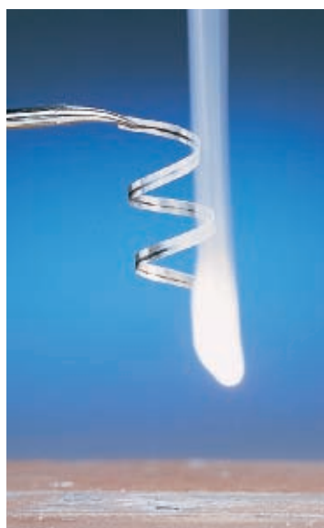
Magnesium burns in air to form MgO and \text{Mg}_3\text{N}_2 .
