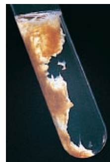
Soluble iron(III) salts form insoluble \text{Fe}(\text{OH})_3 when they are reacted with a hydroxide base.
