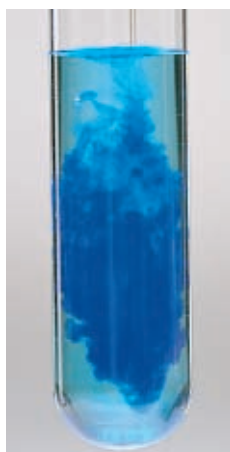
Copper (formation of [\text{Cu}(\text{NH}_3)_4](\text{OH})_2 )
