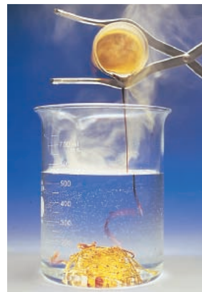
Molten sulfur returns to its orthorhombic form upon cooling.
