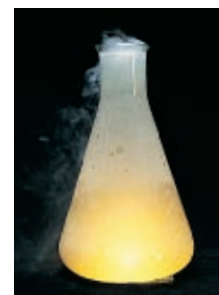
Sodium reacts vigorously with chlorine to produce \text{NaCl} . Most salts of Group 1 metals are white crystalline compounds.
