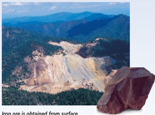
Iron ore is obtained from surface mines. Hematite, \text{Fe}_2\text{O}_3 , is the most common iron ore.
