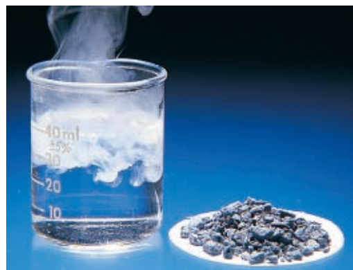
Calcium reacts with water to form hydrogen gas.
